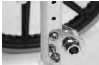
Pic. 1: Wheel assembly mounted on the frame
